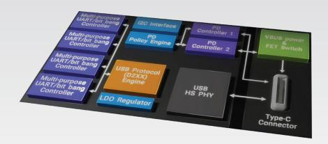
The Power Delivery series has up to two Type-C/PD ports, with PD1 port supporting both power sink and source roles (Initial Sink), and PD2 port only supporting a power sink port role.
