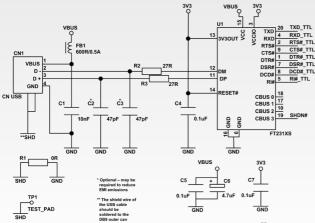
It is possible for the design to simply use RXD and TXD signals but with FTDI solutions the option to implement full modem control is also provided.
